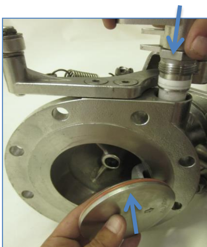
9 - Put the new poppet by pushing the spindle
