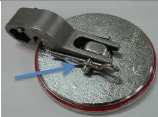
MK4 : (NX3...) : modification of the poppet and pusher
