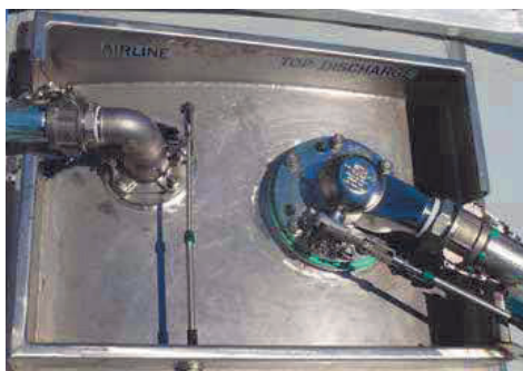
An airline and a top discharge valve operated from ground level thanks to a manual remote control
