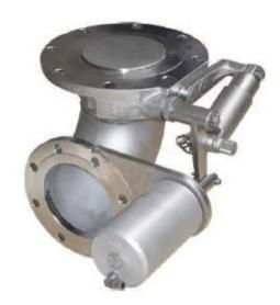
4" CHEMFLOW TM MK2 90° pneumatic or manual footvalve - designed to discharge liquid chemicals and foodstuffs carried in road tankers - The external spring design is perfectly suited to tanks containing viscous fluids and allows easy cleaning and maintenance.
