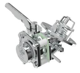
3" NEATCO MKII  $45^{\circ}$  or  $30^{\circ}$  bottom discharge assembly combines one 3" NEATCO™ MKII footvalve, one 3" TANKFLY™ butterfly valve, and one 3" BSP threaded outlet nozzle with cap, all fully assembled together with gaskets and screws - This version improves the flow performance avoiding retention and also improves solidness due to FEA Design. Each bottom discharge is individually tested on a dedicated test bench and has the Perolo guarantee for leak-tightness.
