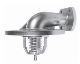
The PEROLO 3" aeration valve allows the venting of the tank to atmospheric pressure during loading and unloading operations. The footvalve operates (open/close) this valve by a cable. This aeration valve opens automatically when the vacuum in the tank is lower than the vacuum setting of the valve.
