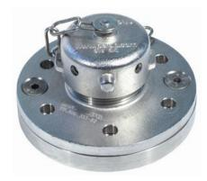
2" H2O2 breather - used on Hydrogen Peroxide tanks to vent the tank during transport - This product is composed by 2 sintered discs. One in the body acts as a filter for the compressed air when pressurizing the tank in unloading operations. In case of tank rollover, the liquid flow rates goes through the second disc. The second disc limits the water flow rate.
