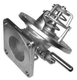
3" NEATCO MKII  $45^{\circ}$  or  $30^{\circ}$  footvalve - designed to be fitted at the bottom of tank containers - no retention, better flow performance - more robust but no heavier - new stuffing box fastening - conical poppet - overall external dimensions reduced allowing more rear cabinet clearances.
