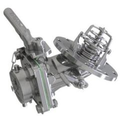
Perolo 3" TWINCO bottom discharge assembly combines one 3" TWINCO  $^{TM}$  footvalve with splined butterfly shaft, and one 3" BSP threaded outlet nozzle with cap, all fully assembled together with gaskets and screws. It is designed to be fitted at the bottom of tank containers. Made of stainless steel 316L/1.4409, this product is suitable for ISO tank containers dedicated to the transport and storage of chemicals and liquid foodstuff.
